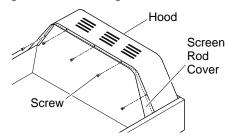
Figure 11 - Removing Hood Screws
